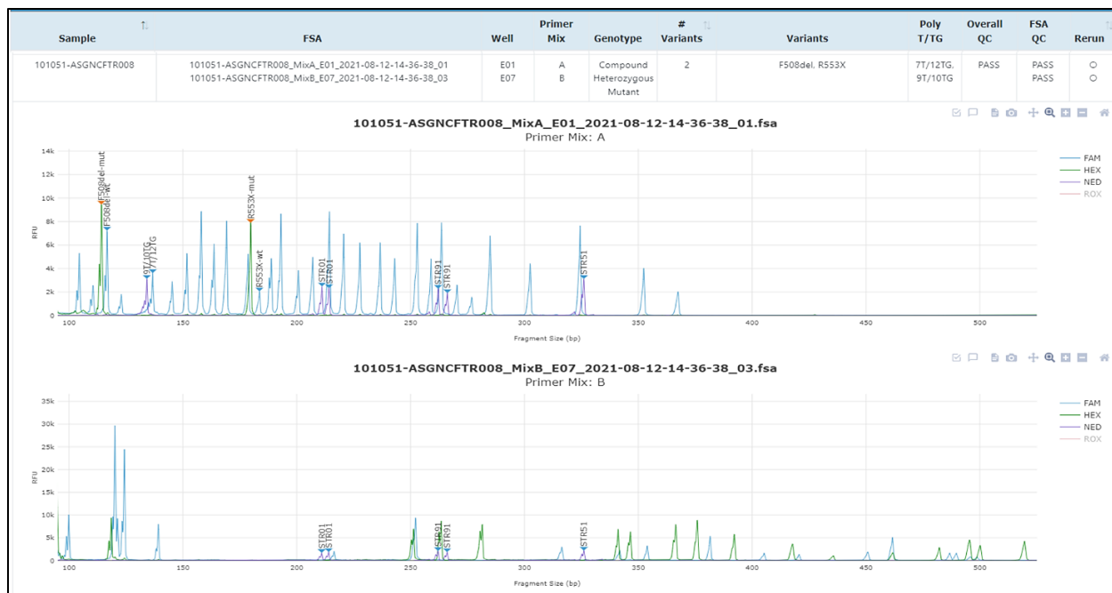
Figure 1. Assay design and example of AmpliDeX® PCR/CE CFTR Kit electropherogram. Allele-specific primers amplify wild type (WT) or mutant (MUT) allele variants with a set of common primers. Amplicons are labeled during amplification and are resolved by CE with detection in the FAM, NED, or HEX channels. The amplicon mobility shift (bp) and/or dye channel differentiates alleles for each variant. CE traces are visualized by overlapping channels in AmpliDeX PCR/CE Reporter with peaks binned based on expected sizes for Primer Mix A and Primer Mix B.
