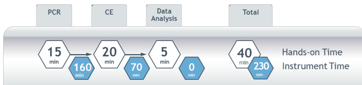
Figure 2. The workflow is streamlined from sample-to-answer and can be performed in less than 5 hours with ~60 minutes of total hands-on time for 12 samples. CE instrument time was documented for a single injection of 24 reactions using an Applied Biosystems 3500xL Genetic Analyzer (24 capillary).
